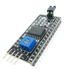
Typically, the controllers are sold with the display and the pair go for around \$2 each direct from China. With this board attached to the Character Display, you can use I2C which requires only 2 pins and power. And you can connect multiple displays.
